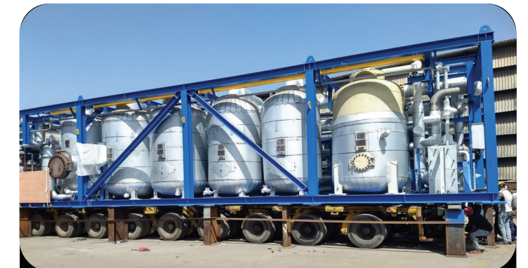
Co2 Purification Plant for Keys California
