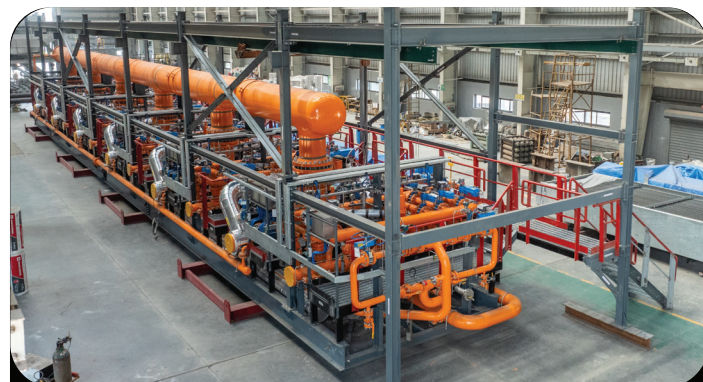
PSA-Skid Package for IOCL
