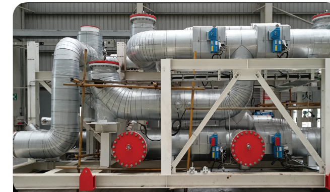
OIL FREE AIR & MOLSIEVE skid for Middle East
